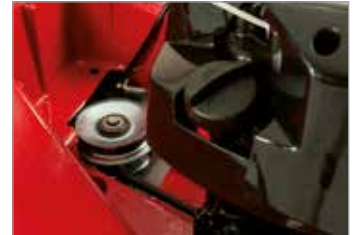
Speed variator pulley for double belt
