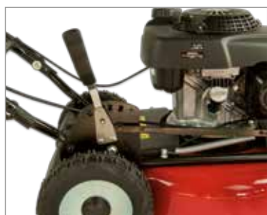
Central height adjustment system and heavy duty carter
