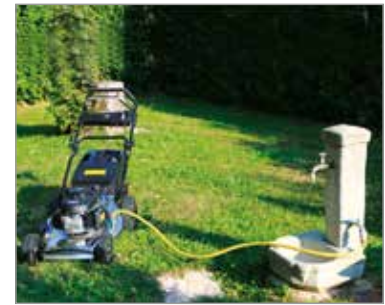
Water connection to properly wash the blade and carter
